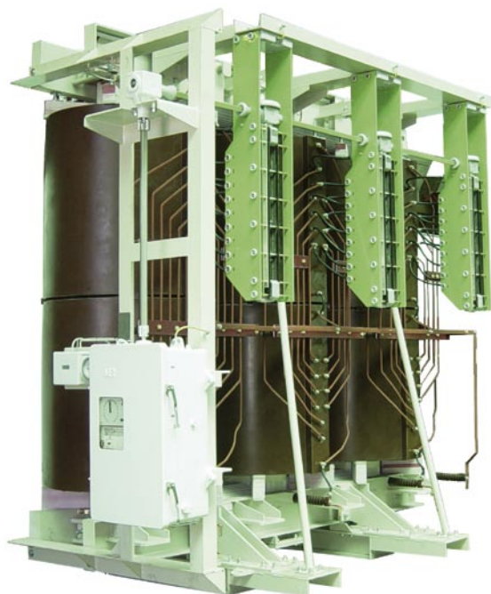
On load tap changer with motor drive for the uninterrupted and automatic adjustment of the transformation ratio under load conditions.
