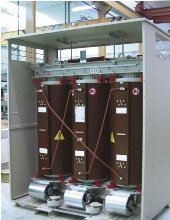
Cooling fans AN/AF (air natural/air forced) transformers refrigerated by fans designed to canalise the air flow into the cooling channels. Up to 50 % capacity increase.
