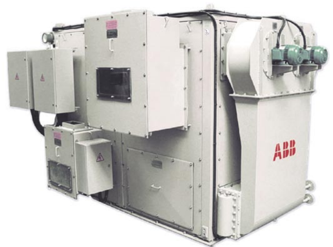
ABB Vacuum Cast Coil dry transformer for marine applications. AFWF (air forced/water forced) cooling by hydrocoolers. Design and manufacturing approved by LLOYD'S Shipping Register, Bureau Veritas, DNV, RINA, ABS
