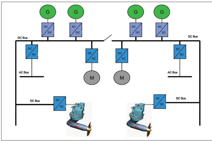
Fig. 4 Onboard DC Grid; Distributed approach.
