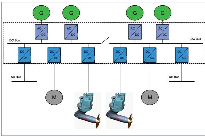
Fig. 3 Onboard DC Grid; Multidrive approach.
