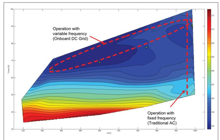
Fig. 5 Engine fuel tests at variable speed (color scheme indicates Specific Fuel Oil Consumption (SFOC) in g/kWh .
