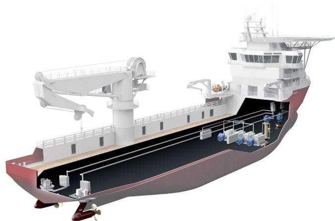
Fig. 1 Platform Supply Vessel with Onboard DC Grid
