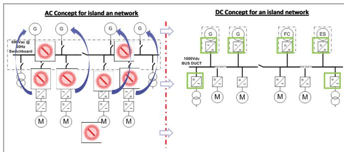
Fig. 2 From AC to DC (single line old vs. new design)
