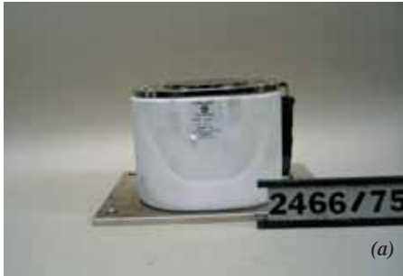
3 Bussmann (a) and Ferraz fuses (b) after one test
