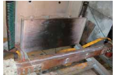
2 High current shunt for calibration measurement
