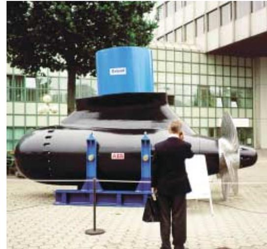
A 1620 kW Azipod unit displayed at SMM98 in Hamburg.
