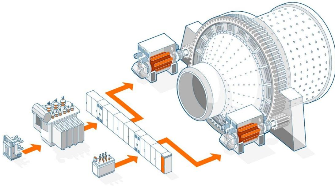
ABB's ring-gear mill drive system
