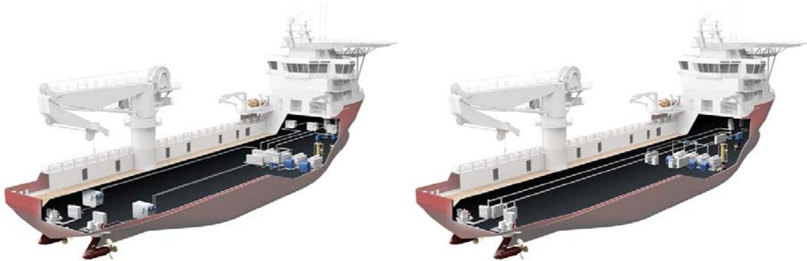
ABB's onboard DC system represents a step forward in optimized propulsion by connecting all DC links and distributing the power through one main DC circuit. It is designed for ships with low-voltage onboard power systems, such as offshore support vessels, tug boats, ferries and yachts, and can reduce fuel consumption and emissions by up to 20 percent.
