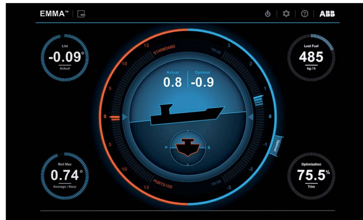
The trim and list optimization display gives a clear indication of the utilized optimization potential. The top right corner indicates a very important performance indicator: lost fuel due to sub-optimal trim.
