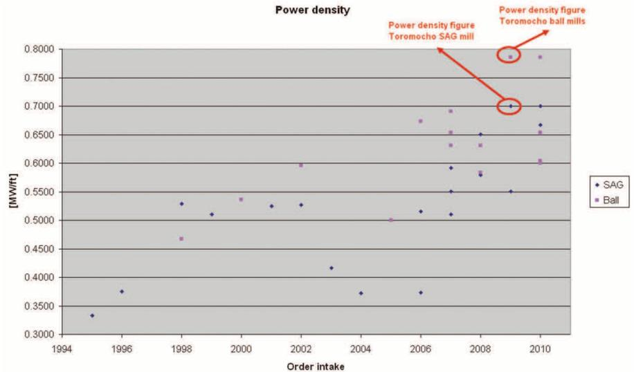
Power density of ABB's Gearless Mill Drives
