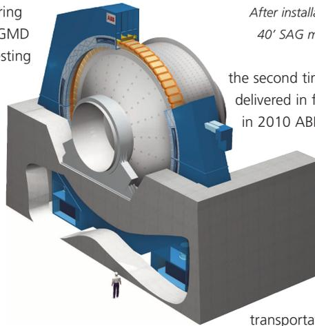
After installation, the stator of a 40' SAG mill is over 21 m high
