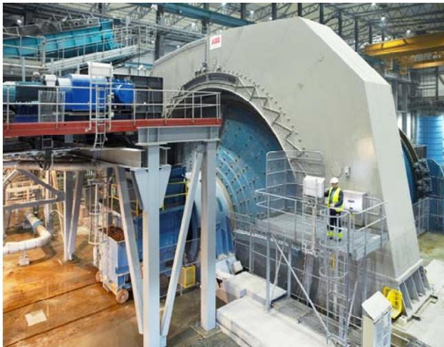
The main component of a GMD is a colossal motor integrated into a drum-like mill in which mineral ore is ground. The motor is equipped with a drive, which starts the mill smoothly without any mechanical stress. The GMDs at Aitik have a rating of 22.5 MW, making them the world's most powerful in operation today. The mills they power are 13.7 meters long and 11.6 meters in diameter, which also makes them the world's largest by volume, and each has a grinding capacity of 2,200 tons of ore per hour.
