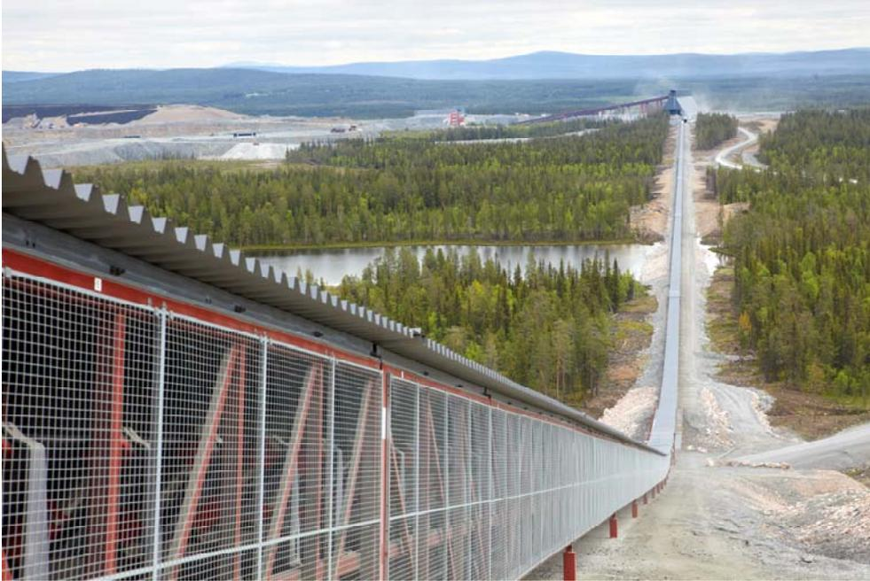
**Caption: A 7 km conveyor driven by ABB motors and drives transports the ore from the mine to the concentrator.**
