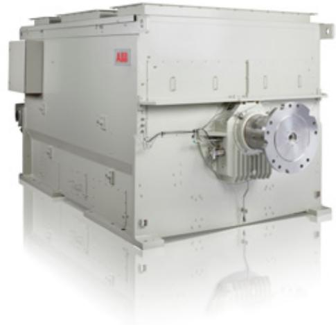
customer requirements, while providing commonly needed features. These state-of-the-art synchronous generators for steam and gas turbine applications feature vacuum pressure impregnation (VPI) of the stator winding system, providing the strength necessary to withstand all mechanical and electrical stresses during operation. The robust stator and the rigid rotor construction - which incorporates solid salient poles - makes the pre-engineered generators extremely reliable.
