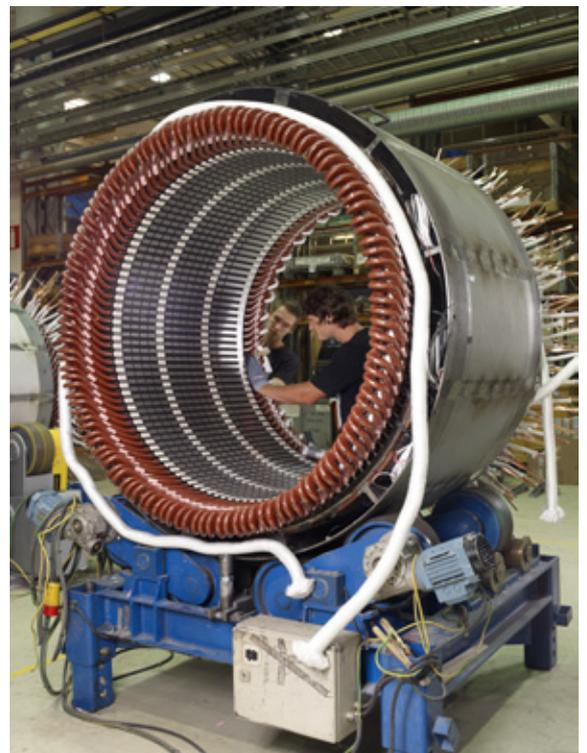
Form wound coils are used for medium or high voltage stators (also available for low voltage stators). High voltage coils include a semiconducting layer to decrease the electrical field at the slot surface.
